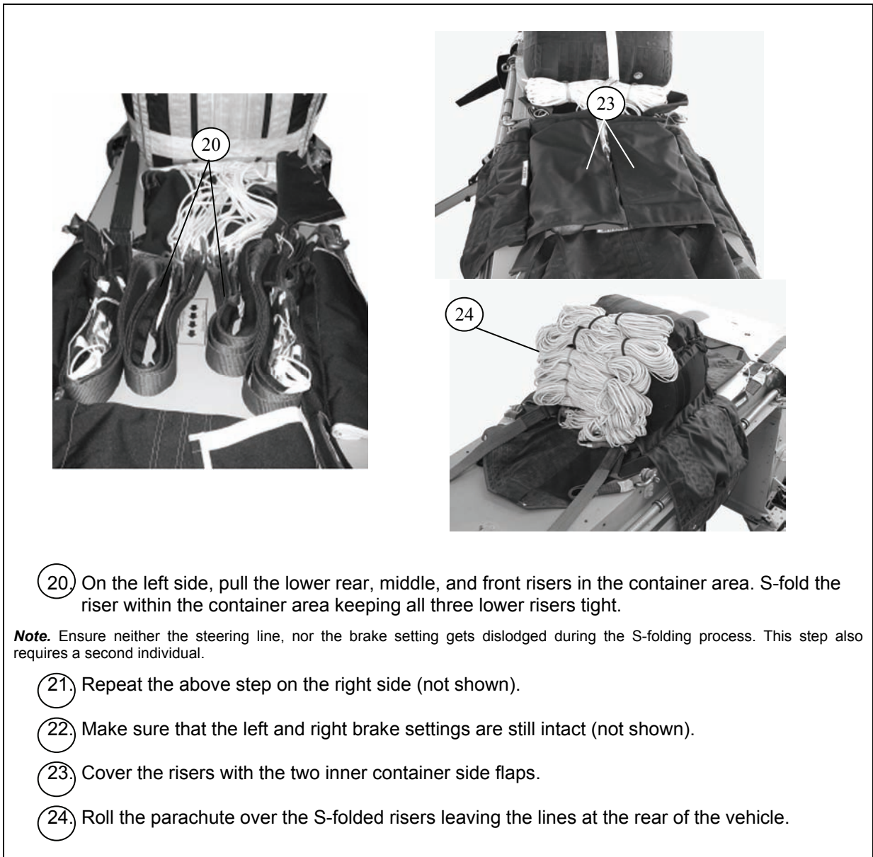
Figure 6-2. Air Launch Parachute Installed (Continued)
